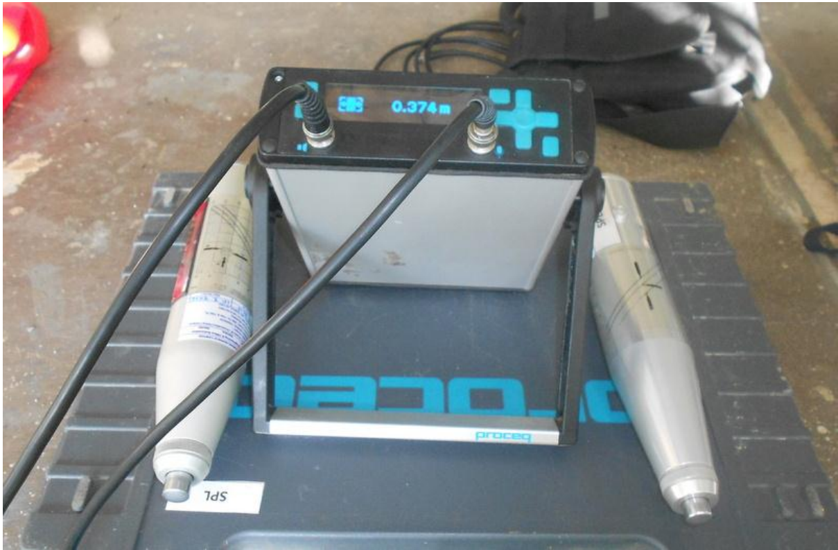
Ultrasonic Pulse Velocity Testing Machine and Rebound Hammer
