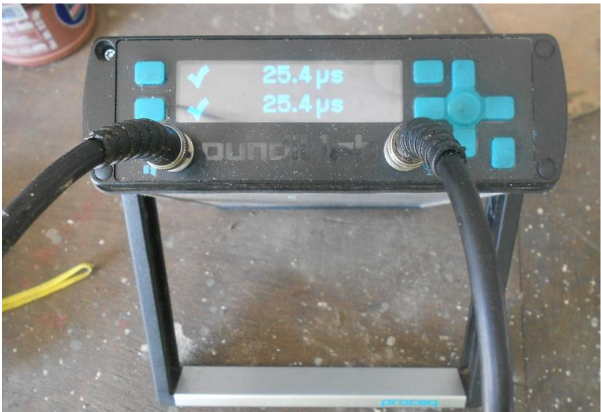
Calibration before UPV Testing
